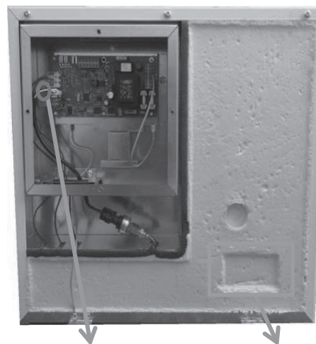
BT15 connector Insulation BT15 is in the back.
