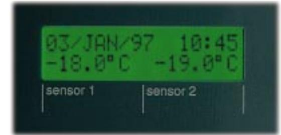
**Back-lit LCD display that allows the display of the recorded data even in poor light conditions.**
